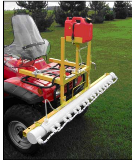
Rope wick applicator for tall weeds
